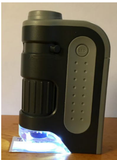
Fig. 9 Mini microscope used for observation of ink/substrate specimens
