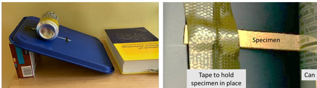
Fig. 19 Setup for the “roll test” using a thin strip of tape and a soda can roller
