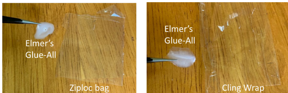
Fig. 13 Photos of Elmer’s Glue-All (completely dry) on polyethylene from cling wrap and a Ziploc bag. The dry adhesive was easily recovered as a film from the cling wrap and Ziploc bag specimens demonstrating adhesive failure (“failed to adhere to substrate”).
